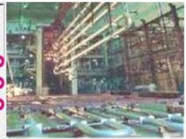
One System (Steam Generator) (2.25 Cr – 1 Mo) with seven core pipes with common envelop – see cross section (fabricated by M/s BHEL, Trichy )
